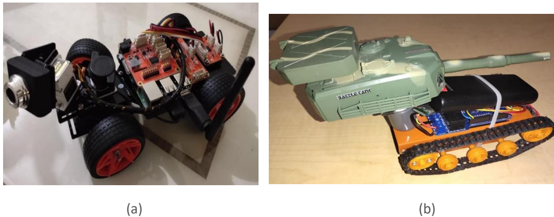
Figure 2. Prototypes of military robot using Wi-Fi technology (a) and bluetooth (b) for controlling the robot. We can control the camera using 2 servos.
